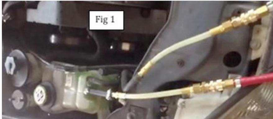
3. Attach the appropriate sized hose (from the Degas adapter kit) to the Degas tank and tighten the worm gear clamp. Connect one of the Degas hose assemblies to the hose now connected to the Degas tank and tighten the worm gear clamp. Connect the unit's RED/ used coolant hose to Degas hose assembly adapter see figure 1.
