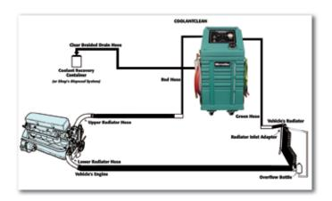
The flush and lubricant process starts from the radiator through all the cooling systems fluid lines and into the water pump.
